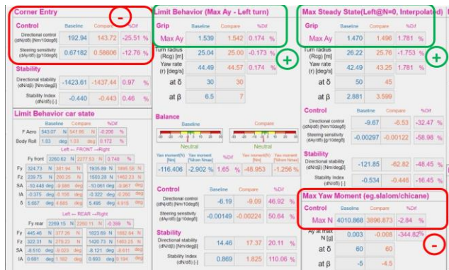
Fig. 21: Result KPI from during designing of Ackermann geometry with baseline being previous year car design
